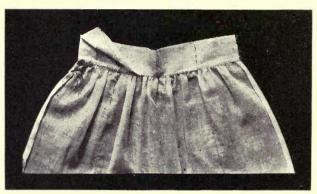
Fig. 40.—Detail of Sewing a Band to Garment
